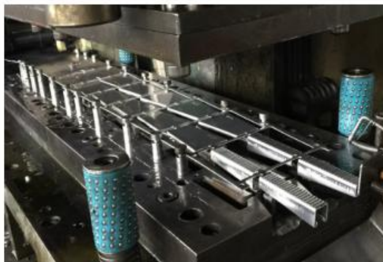
Drop wire clamps are produced by stamping process.
